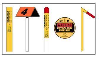
Markers and warning signs only indicate the general location of a pipeline. They cannot be relied upon to indicate the exact position of the pipeline they mark. Also, the pipeline may not follow a straight course between markers. And, while markers are helpful in locating pipelines, they are limited in the information they provide. They provide no information, for example, about the depth or number of pipelines in the vicinity.
