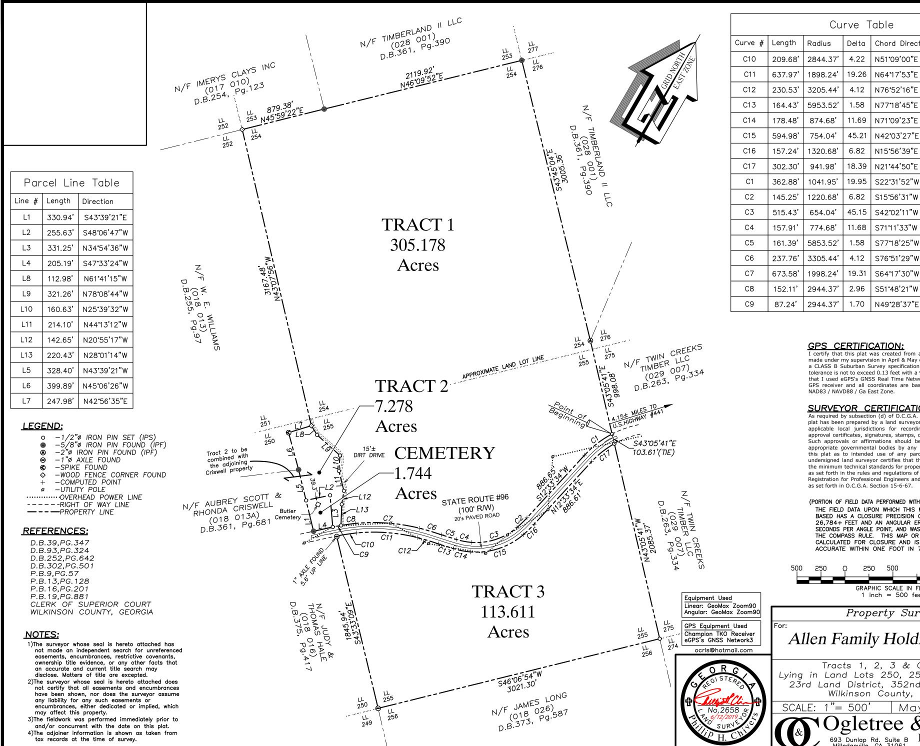
Chord Length Chord Direction N51°09'00"E 209.63 N64°17'53"E 634.97 N76°52'16"E 230.48 N77°18'45"E 164.43' N71°09'23"E 178.17 N42°03'27"E 579.67 N15°56'39"E 157.15 N21°44'50"E 301.01 S22°31'52"W 361.05 S15°56'31"W 145.16' S42°02'11"W 502.20 | S71°11'33"W 157.64 S77°18'25"W 161.38' 237.71 S76°51'29"W S64°17'30"W 670.40 S51°48'21"W 152.09'
