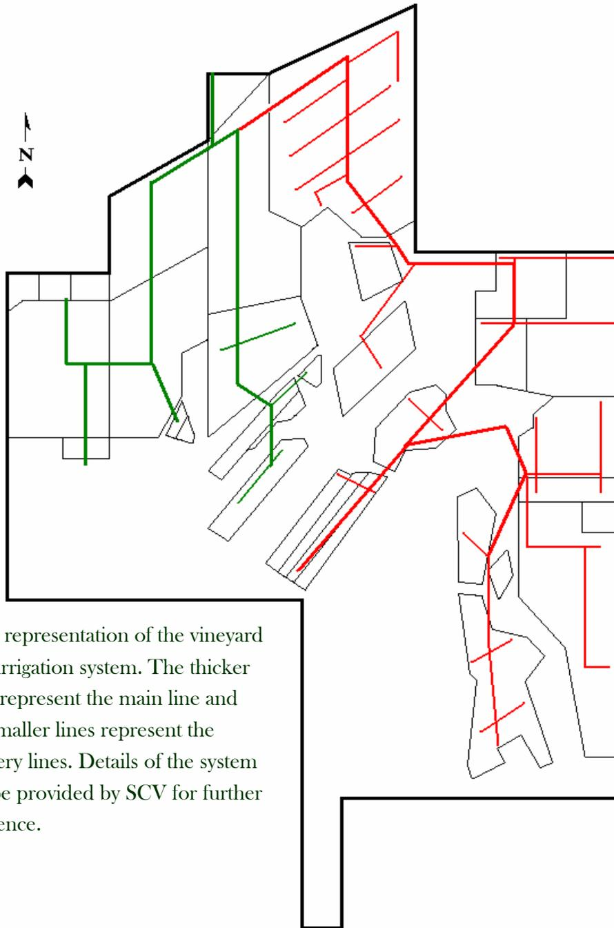
Basic representation of the vineyard drip irrigation system. The thicker lines represent the main line and the smaller lines represent the delivery lines. Details of the system can be provided by SCV for further reference.
