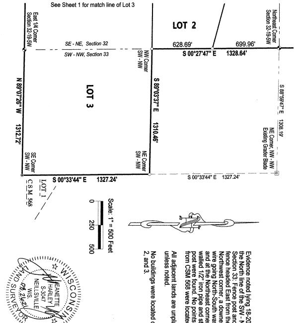
Northwest corner, a downed fence wire going North-South was right on, and at the Northeast corner an thin walled 1/2" iron pipe and steel fence post were found. No points on line from CSM 568 were located. Evidence noted lying 18-20' South of the North line of the SW - NW, Section 33: Fence post and partial fence headed East from the
