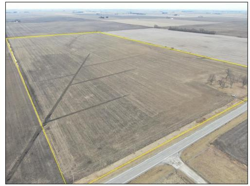
Looking northeast from IL Route 9 at southwest corner. The lines are surface drains installed to relieve any surface water buildup on the farm. The main tile lines are tied into neighbor's tile, receiving that water as well. Surface drain installed post-harvest 2022. (Information from former tenant.)
