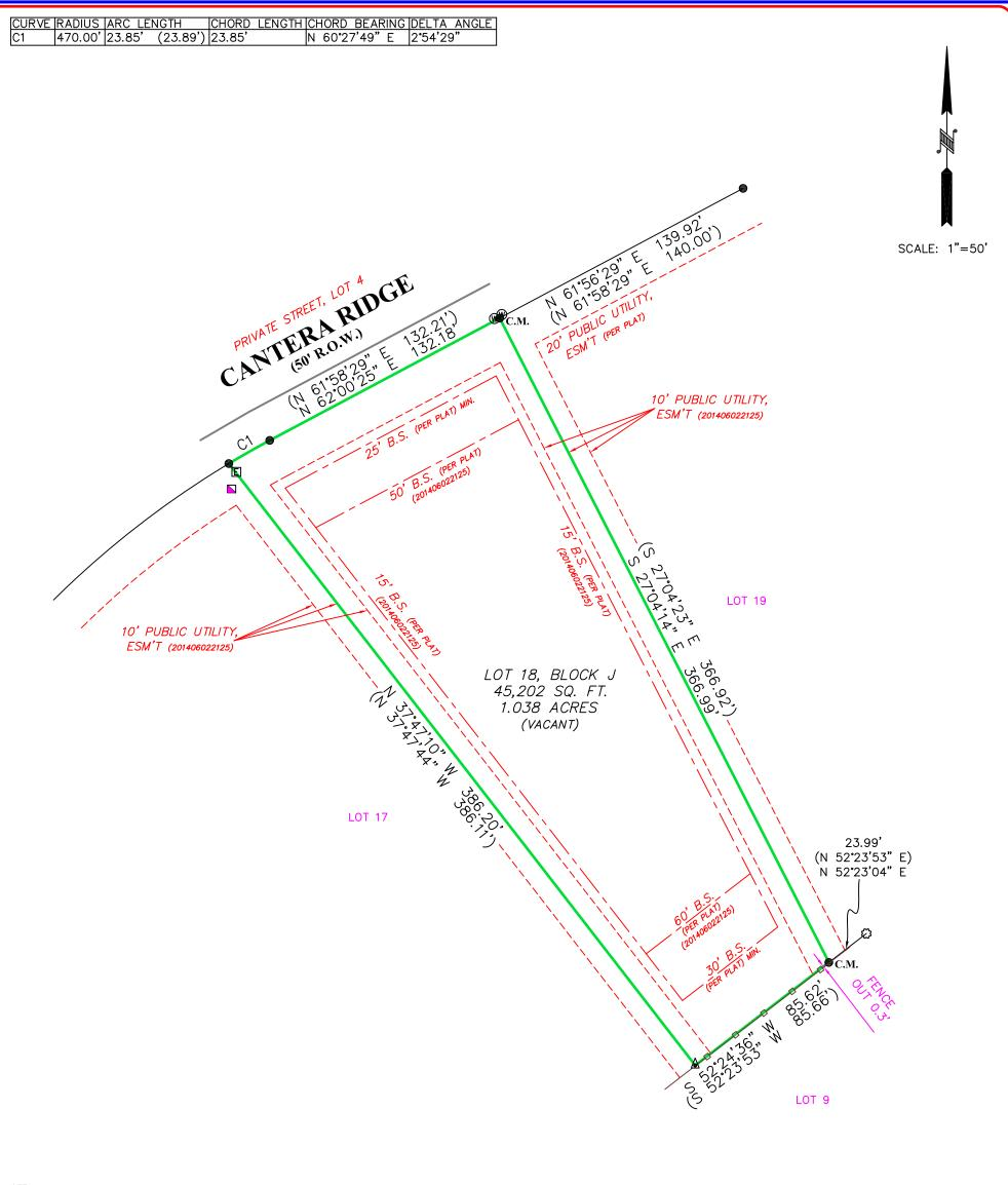
Bearings shown hereon are based on actual GPS Central Zone, Grid.
