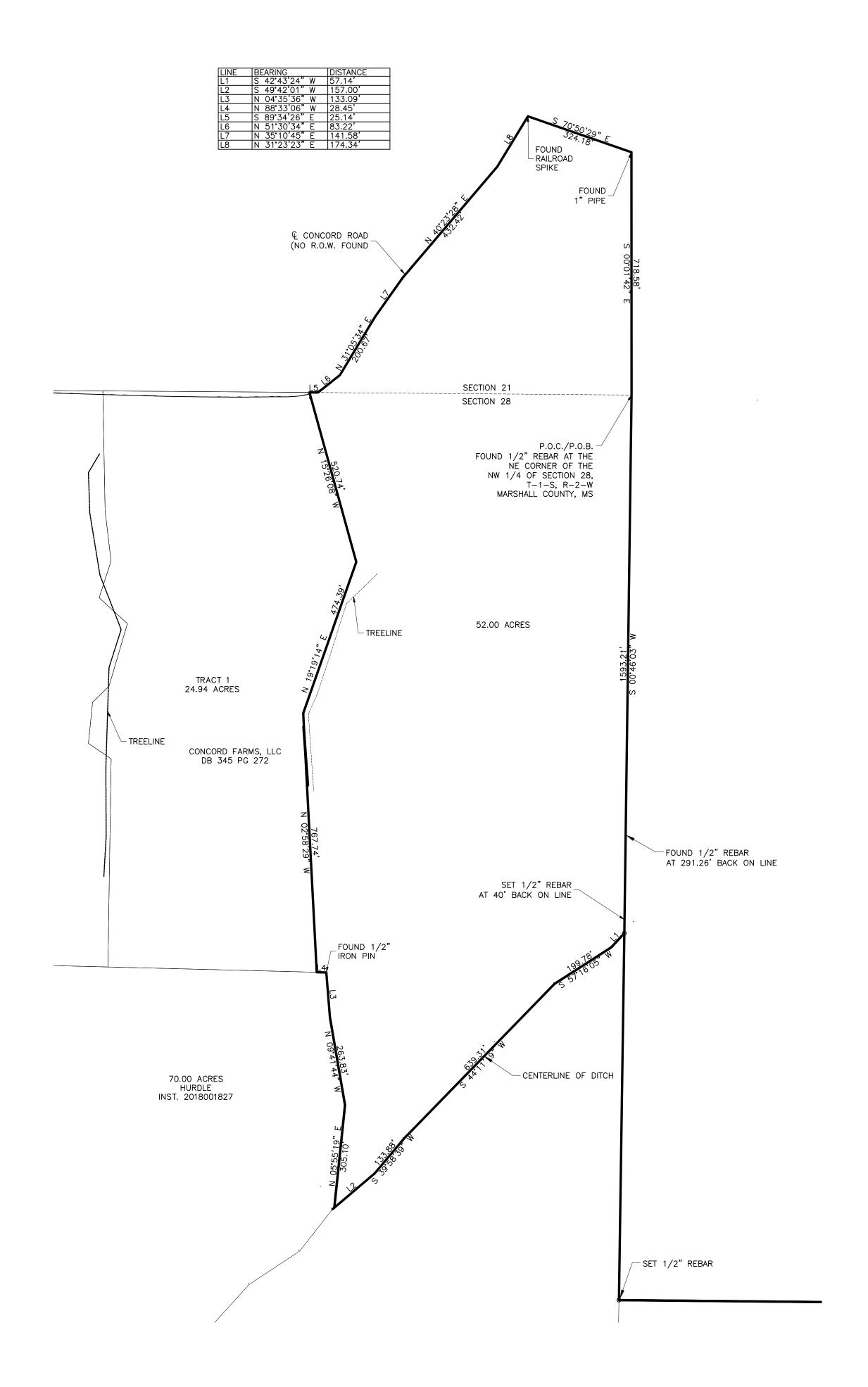
GRID BEARINGS SHOWN ON THIS PLAT. SURVEY PERFORMED BY CONVENTIONAL METHODS. GPS CONTROL SET USING GCGC RTK NETWORK. AZIMUTH ORIENTATION IS FROM ZERO GRID NORTH.
