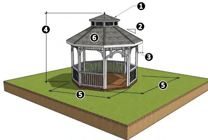
❶ CUPOLA OR CLERESTORY; ❷ 2:1 MINIMUM ROOF PITCH; ❸ 1.5-FOOT MAXIMUM OVERHANG; ❹ 15-FOOT MAXIMUM HEIGHT WITH OR WITHOUT A CUPOLA OR CLERESTORY; ❺ 12-FOOT MAXIMUM; ❻ ROOF MATERIAL SHALL BE METAL. (Image from City of Rockwell UDC Ordinance 21-01)
