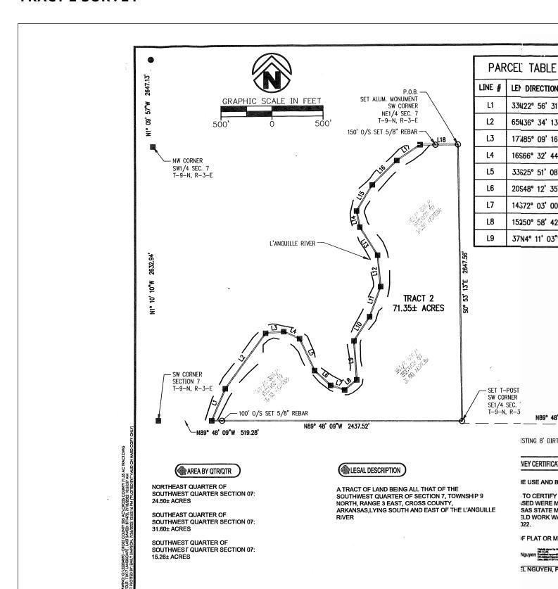
PARCEL LINE TABLE LINE # LENGTH DIRECTION N33° 29' 34"E L10 275.30 N20° 25' 31"E L11 306.91 L12 300.14 N5° 47' 41"W N32° 11' 31"W L13 321.82 L14 158.02 N11° 38' 35"W N31° 40' 30"E L15 293.28 L16 332.84 N45° 24' 09"E L17 271.04 N56° 26' 09"E L18 368.42 N89° 54' 36"E
